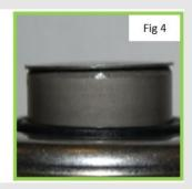
The piston retaining ring has no deformation or rippling. This shows that the cylinder has not been overstroked.
